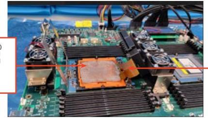
FFED into SP5 test socket – flex cable exit shown
