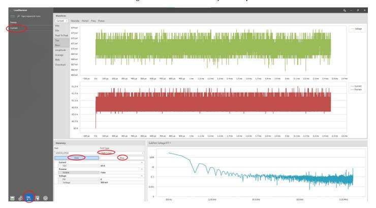
Custom **dynamic** test - starts with selecting **slam** and runs continuously until **stop** is activated.
