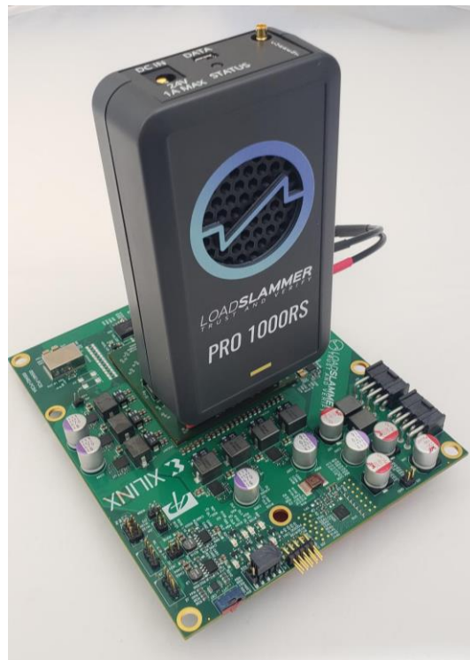
Fig. 1. LoadSlammer Pro1000RS connected to DUT.
