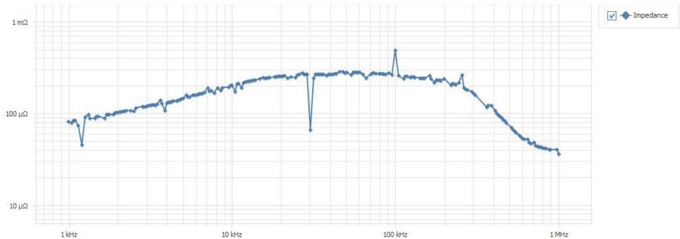
Fig. 10. Impedance measurement with a 20-A offset and a 40-A amplitude.
