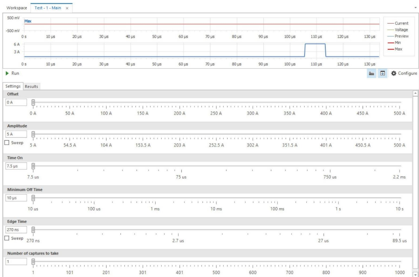
Fig. 2. LoadSlammer settings for a step-load test on the DUT.
